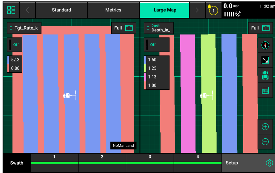
Figure 2. Tractor display screen showing simultaneous implementation of variable seeding rate (zero or 52,300 seeds per acre) and seed trench depth (1, 1-1/8, 1-1/4, and 1-1/2 inches).
