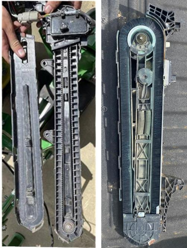
Figure 3. Internal views of Ag Leader Technology's SureSpeed® flighted belt (left) and John Deere's ExactEmerge™ brush belt (right) seed delivery systems.
