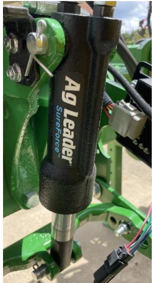
Figure 3: Hydraulic downforce system.
