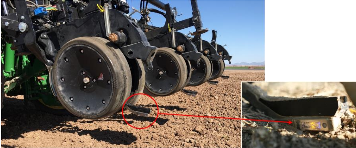
Figure 6. Precision Planting SmartFirmer with a closeup of the sensor shown to the right.
