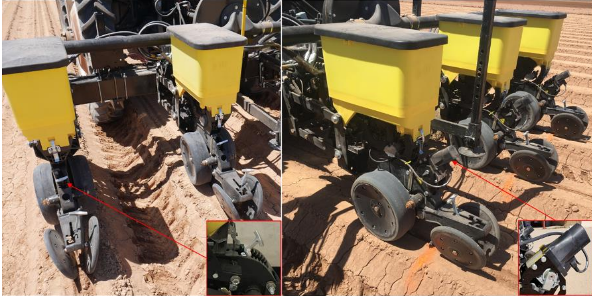
Figure 4: John Deere MaxEmerge row units with manual mechanical depth setting (left) and retrofitted with electric drive (right).
