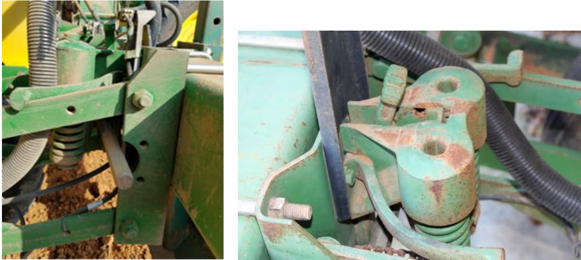
Figure 1: Mechanical (spring) downforce system. Left image is the sideview of the spring mechanism and the right photo shows the T-bar handle used change spring tension.
