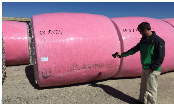
Figure 1. An android app can be paired with a hand-held scanner to read the RFID tags on the cotton modules.
