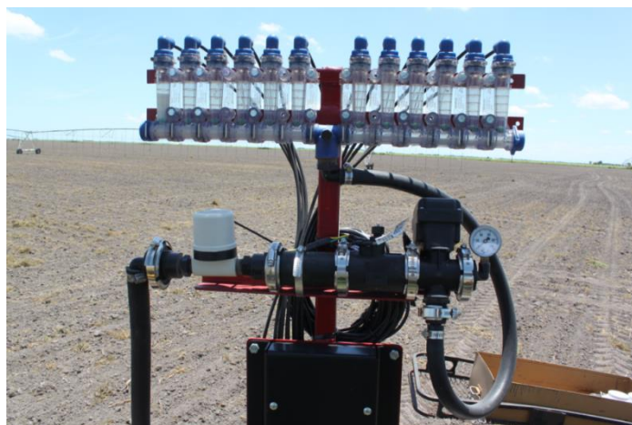
Figure 6. A variable rate control system consisting of a controller, a servo valve, a flowmeter, and a shutoff valve integrated to a John Deere tractor equipped with John Deere GS2 Display and StarFire RTK GPS.
