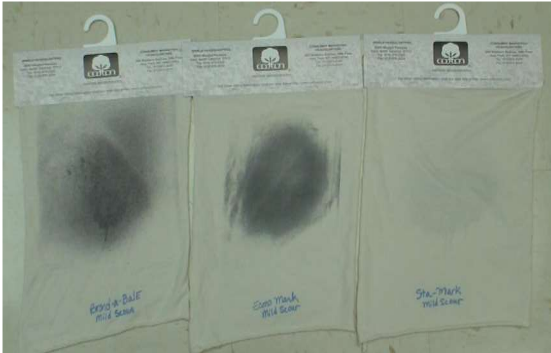
Figure 2: Sprayed fabric after mild scour using soda ash (Left to Right: BRAND-A-BALE®, ECONO-MARK, STA-MARK®)
