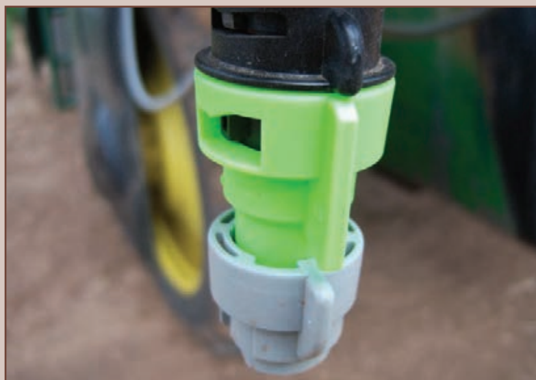
Figure 7. A TurboDrop variable orifice nozzle by Greenleaf. The green portion contains the variable orifice for metering and the grey portion is the flat fan tip to create a pattern.
