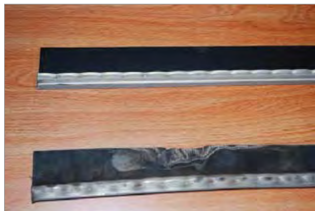
New bat (top) and worn bat (bottom).
