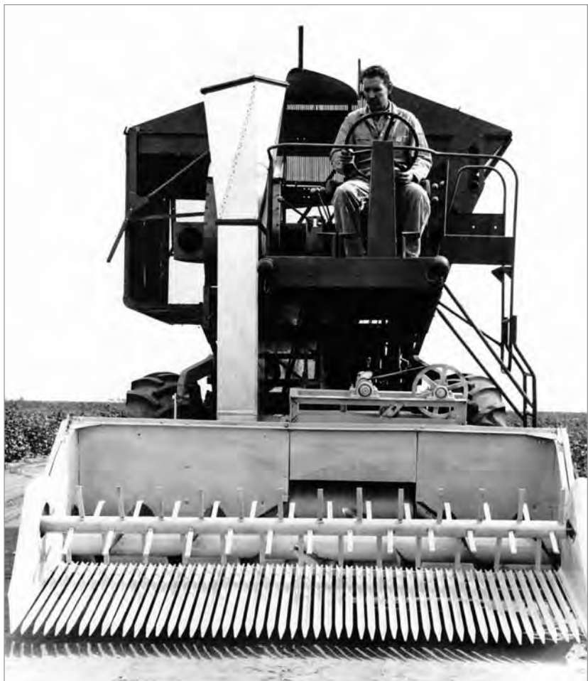
Cotton harvesting machine configured with a finger stripper header (about 1963).
