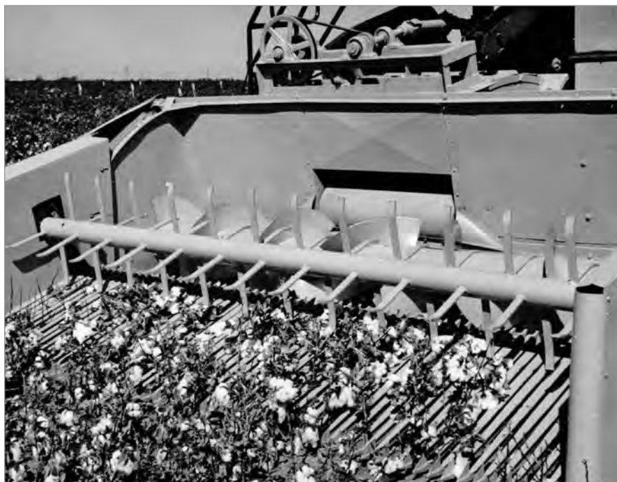
Cotton harvesting machine configured with a finger stripper header (about 1963).
