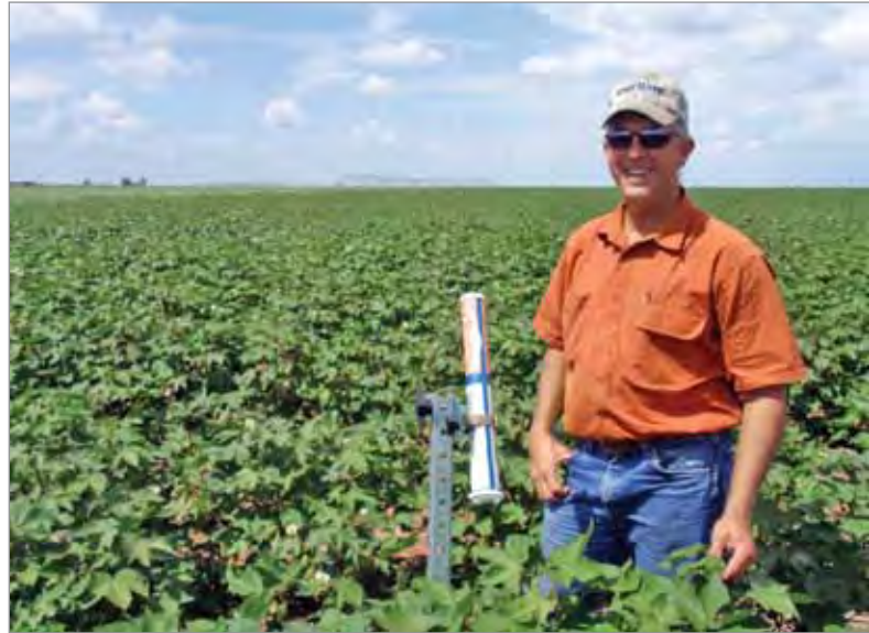
Figure 6.2 – West Texas farmer inspecting an infrared thermometer used to monitor canopy temperature.
